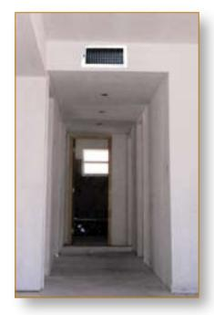
The effect of the lower ceiling height can be offset by increasing the hall width (right).
