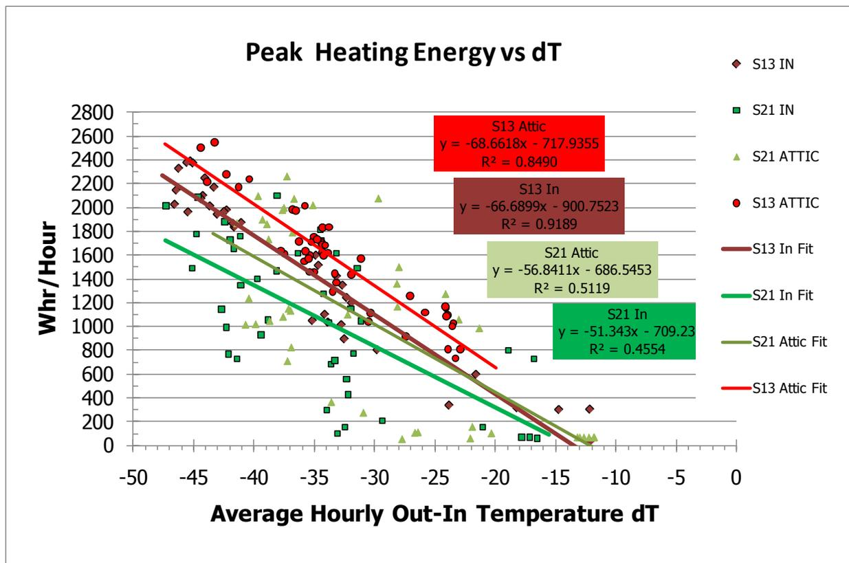
Figure 10. Least-squares best-fit regression analysis for the hours of 2 to 8 AM from cold winter days for four experimental configurations.
