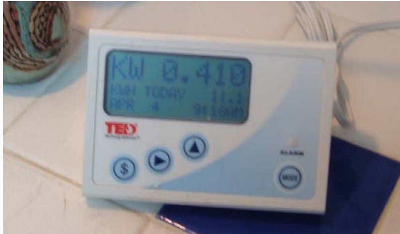
Figure 1-11 TED The Energy Detective
