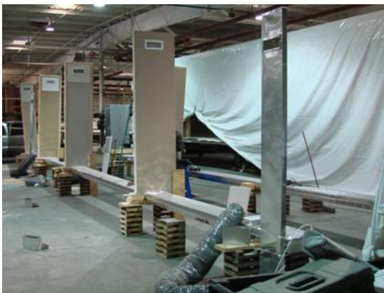
Figure I-2 Floor duct system with high side discharge outlets under construction being tested with duct tester
