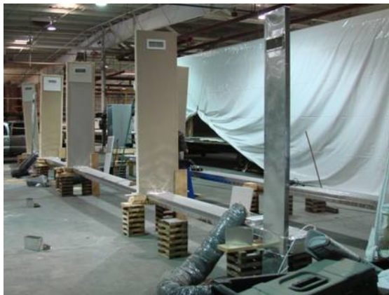
Figure 1-1 Floor duct system with high side discharge outlets under construction being tested with duct tester
