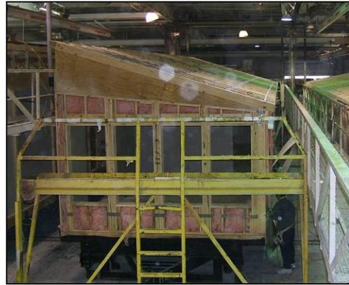
**Figure 58** Palm Harbor HUD Code Manufactured Housing factory – production line.
