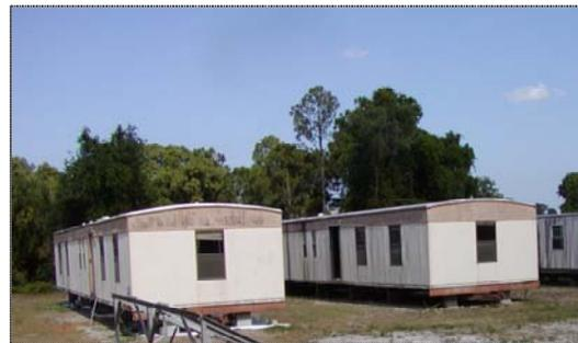
**Figure 81** The test units in place. Note white ground cover under unit on left, exposed dirt under unit on right.
