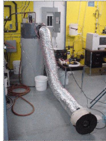
*Figure 112 Airflow measurements using a Duct tester on heat pump cold air discharge side.*
