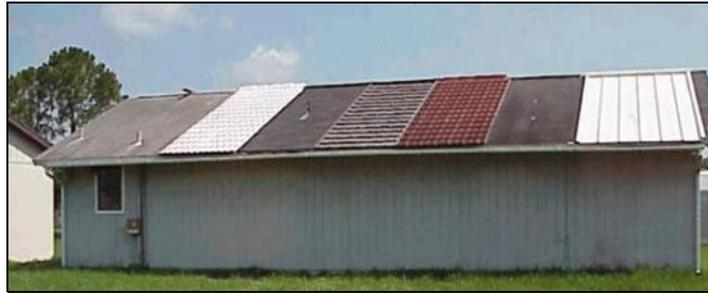
**Figure 106** 2001 Experimental roof cell. Cells are numbered from left to right starting with the cell second in from the left.
