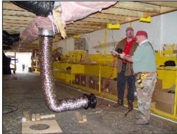
*Figure 52 Southern Energy Homes quality control engineer conducts in-plant duct leakage test.*
