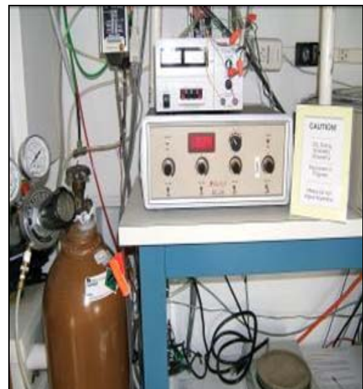
Figure 5 Carbon dioxide tank and dispenser
