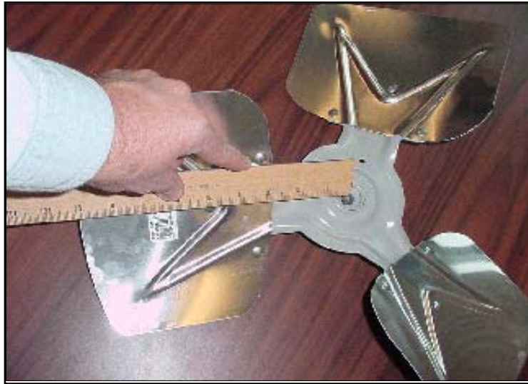
Figure 2. Stamped metal condenser fan blades for a 3-ton condenser
