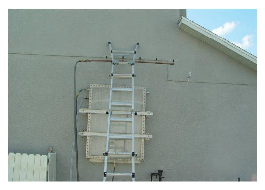
Figure 50 Spray rack mounted above test chamber – note rain gauge to right of spray rack
