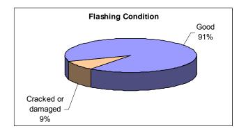
Figure 39 Condition of flashings in homes that leaked
