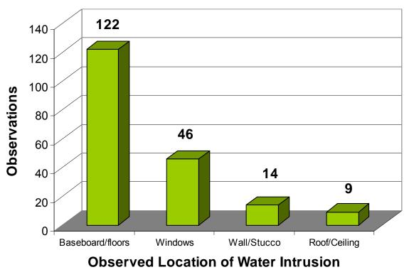
Figure 8 Respondent profile by observed location of water intrusion
