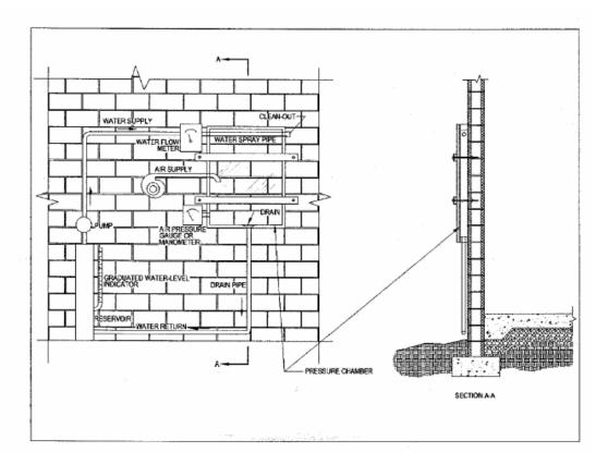
Figure 12 Schematic of test equipment and setup (ASTM 1601 - 04 2004)
