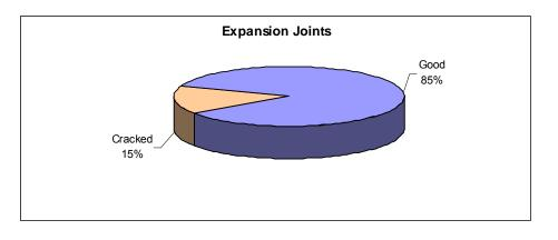
Figure 40 Condition of expansion joints in homes that leaked
