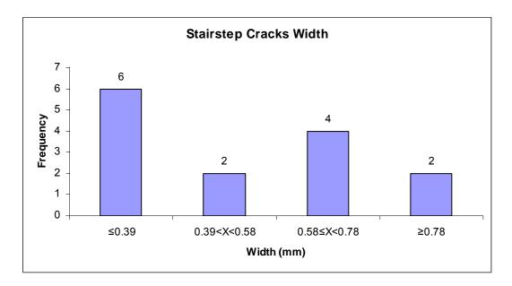
Figure 45 Typical stairstep crack width in homes that leaked
