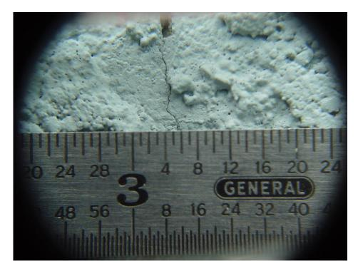
Figure 33 Typical crack less than 0.39 mm (1/64 inch) wide
