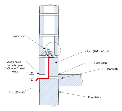
Figure 67 Flashing details for masonry construction (adapted from TEK 19-5A 2003)
