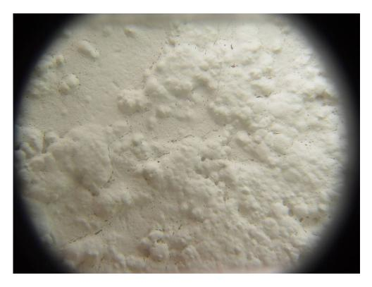
Figure 31 Tiny micro-cracks in stucco seen through 5X jeweler's loop
