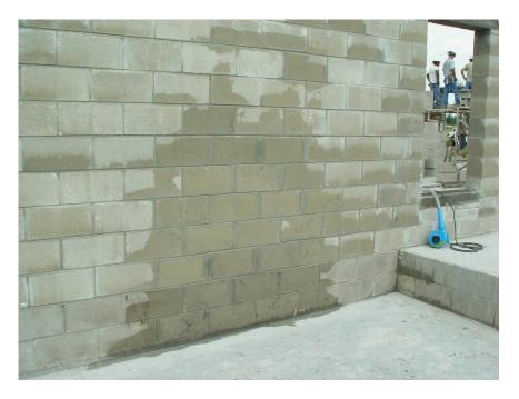
Figure 16 Dampness on inside of wall during test
