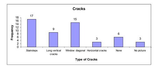
Figure 44 Cracks observed in homes that leaked
