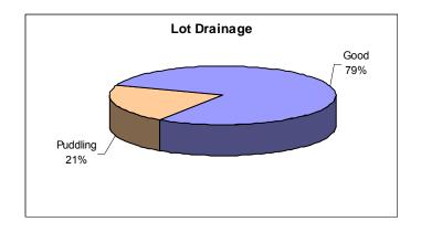
Figure 46 Condition of lot drainage in homes that leaked
