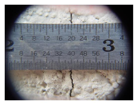
Figure 37 Typical crack between 0.58mm (1/48 inch) and 0.78 (1/32 inch) wide
