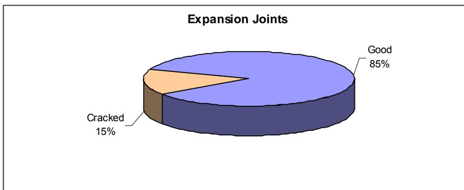
Figure 40 Condition of expansion joints in homes that leaked
