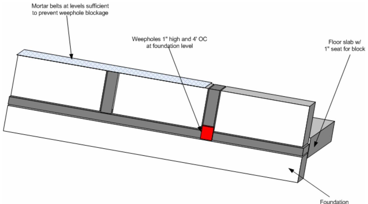
Figure 66 Weephole concepts in concrete block wall
