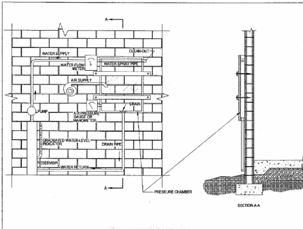
Figure 12 Schematic of test equipment and setup (ASTM 1601 - 04 2004)
