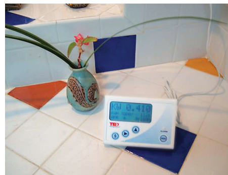
Free standing display of The Energy Detective (TED) shows that the house is drawing 0.4 kW.
